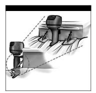
Bennett Trim Tabs are attached to the bottom edge of the transom. When the helm control is pressed, the trim tabs move into position. Water-force on the trim tab surface creates upward pressure, raising the stern and lowering the bow. Properly sized trim tabs improve the performance of your boat in a wide range of weight, weather and water conditions.
