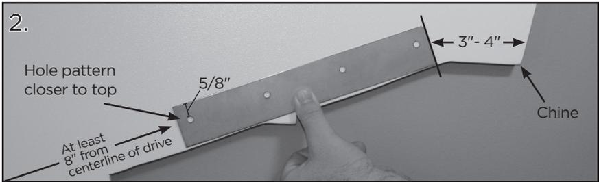
**Position the Tab.** Using the backing plate, choose a location 3-4" from the chine. Maintain a minimum of 8" from the centerline of your drive unit to the closest edge of the trim tab. Align the bottom of the backing plate flush with the bottom of the transom. The hole pattern on the backing plate should be closer to the top edge of the backing plate.
