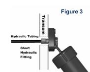
Step 4 Remove upper hinge from transom and remove pipe nipple. If you have a short fitting use a 7/16" wrench to remove it from the upper hinge.
