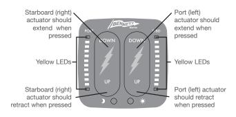
If either of the upper yellow LEDs is flashing, try to move the actuator using the control to confirm that there is a problem.
