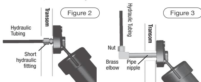
**Step 2** - Outside the transom, unscrew and remove the actuator away from the transom. Remove the pipe nipple.
