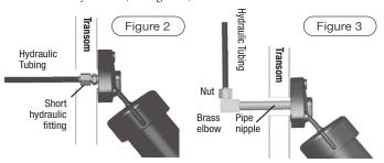
**Step 2** - Outside the transom, unscrew and remove the actuator away from the transom. Remove the pipe nipple.
