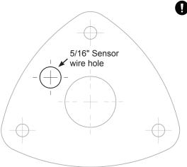
Please note that a sensor hole is only required for sensor-equipped upper hinges. If your upper hinge does not have sensor wires, do not drill the sensor hole.
