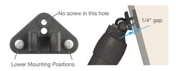
Pull the excess cable through the transom leaving enough cable to prevent the actuator from binding during its normal movement.
