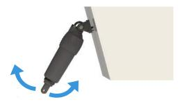
Apply 3M 5200 waterproof sealant on the mounting surface and around the wiring of the new actuator.
