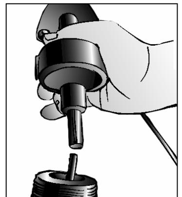
**Step 7** Cover end of pipe nipple with masking tape. Apply sealant to actuator upper hinge surface around pipe nipple, screw holes, and cable. Feed actuator cable through 5/16" hole and secure actuator upper hinge to transom with mounting screws. Grasp cylinder body with both hands and tighten (clockwise) securely. Repeat for other side. Run cables to helm.
