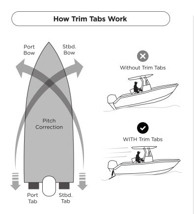
When the tabs are deployed downward, the water force on the trim tab surface creates upward pressure, raising the stern and lowering the bow. The port trim tab lowers the starboard side bow, and the starboard trim tab lowers the port side bow.
