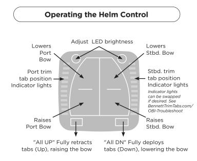
Trim tabs are easy to use. After just a few times using, tab operation will become second nature. The concept is simple but the results are impressive.
