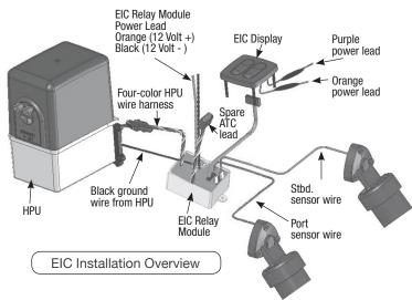
**Step 10** - **Mounting the EIC Relay Module.** The Module is best located in a dry location close to the Hydraulic Power Unit. Use the mounting hardware to secure it in place.
