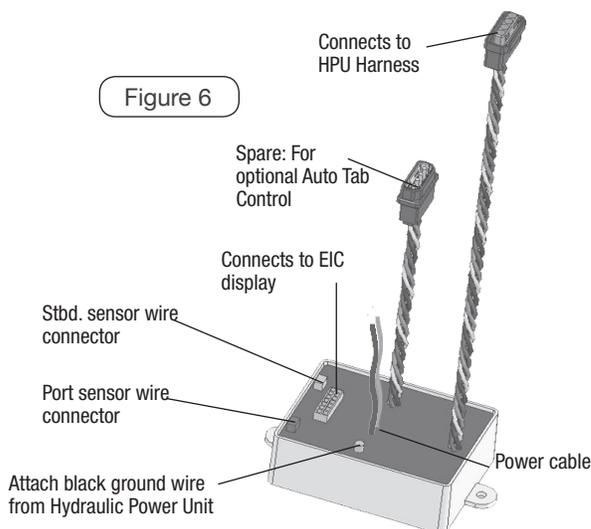
**Ground wire from pump:** Run the black ground wire from the back of the hydraulic power unit to the grounding stud on the Relay Module. Crimp the supplied ring terminal on wire and secure with 10-32 hex nut.
