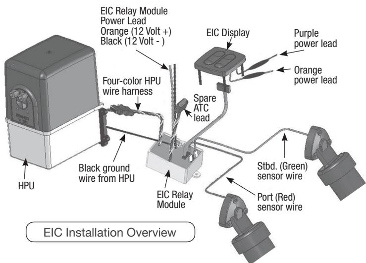
**Step 10 - Mounting the EIC Relay Module.** The Module is best located in a dry location close to the Hydraulic Power Unit. Use the mounting hardware to secure it in place.
