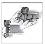
Bennett Trim Tabs are attached to the bottom edge of the transom. When the helm control is pressed, the trim tabs move into position. Water-force on the trim tab surface creates upward pressure, raising the stern and lowering the bow. Properly sized trim tabs improve the performance of your boat in a wide range of weight, weather and water
