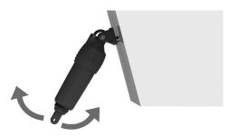
Apply 3M 5200 waterproof sealant on the mounting surface and around the wiring of the new actuator.
