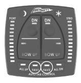
start automatic operations, the unit must have the FAV position set (see "Setting a Favorite Position" on page 37), and the initial set-up described on page 23 must have been already performed.
