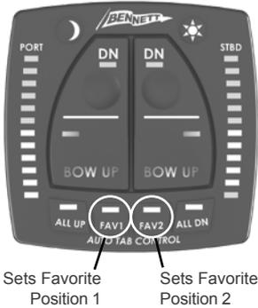
The ATP Helm Control allows for the user to set two different favorite positions. These positions are a combination of pitch and roll attitudes that the user feels are comfortable or useful running attitudes for the boat.
