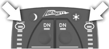
detect the presence of sensors in the actuators. Check to make sure the red and green sensor cables are connected to the ATP Control Unit. If the system does not have actuator sensors, skip to page 22.
