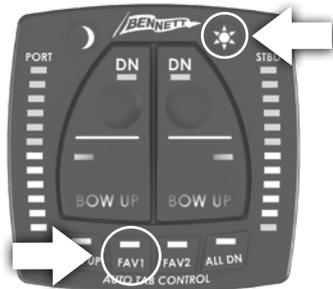
mode. The four yellow LEDs will blink to let you know that the system has gone into orientation mode. The system will now look for an acceleration due to the boat starting. This must be the next acceleration that the boat experiences. Throttle up to speed without using trim tabs. The
