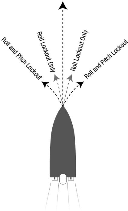
boat is in a turn and modify the way that it tries to adjust. If the turn is fairly gradual (less than 1 degree per second) the ATP control will still make adjustments to the boat to compensate for pitch changes. These pitch changes are uniform on both
