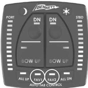
start automatic operations, the unit must have the FAV position set (see "Setting a Favorite Position" on page 37), and the initial set-up
