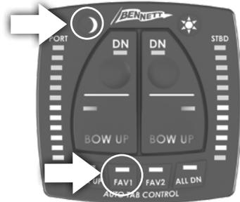
button and the FAV1 button at the same time for at least 5 seconds (or longer which will calculate the average measurement during that span of time).
