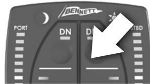
port actuator should extend. If the port actuator does not extend, or the starboard actuator extends instead of the port actuator, refer to the troubleshooting section on page 44.
