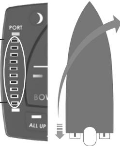
The red LEDs represent the actual movement of the tabs. As the tabs move from the full-up position to the full-down position the red LEDs will illuminate to illustrate the trim tab
