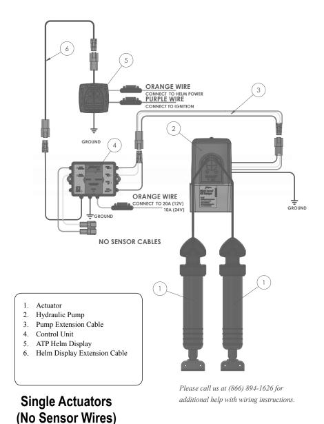
**Please note:** Trim tab position indication will not work with this setup. See page 10 for setup with indication. To add sensors see BennettTrimTabs.com /ATPSensors
