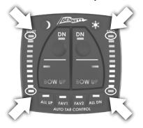
Press and hold both BOW DN buttons until both actuators fully extend. The red LEDs on the display should show the actuator position as the actuators deploy.
