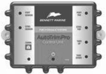
The ATP Control Unit is the sensor and processor for the ATP system which activates the hydraulic pumps that run the trim tabs. The unit contains an accelerometer, gyroscope, and an electronic
