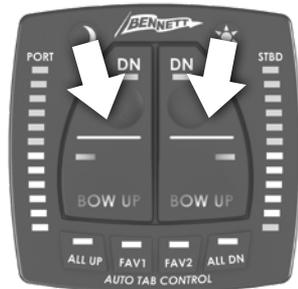
8. Press and hold both BOW UP buttons until both actuators return to the full-up position. The red LEDs on the display should show the actuator position as the actuators retract.
