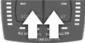
6. Once calibration is complete, the four yellow LEDs in the corners should be continuously on.
