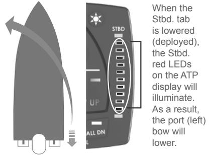
No red LEDs illuminated indicates that the tabs are fully retracted (up). If the red LEDs are flashing, the system does not have a calibration stored for the position display. See page 20 for calibration instructions.
