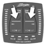
8. Press and hold both BOW UP buttons until both actuators return to the full-up position. The red LEDs on the display should show the actuator position as the actuators retract.
