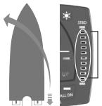
When the Stbd. tab is lowered (deployed), the Stbd. red LEDs on the ATP display will illuminate. As a result, the port (left) bow will lower.
