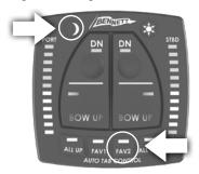
Moon and FAV2 buttons for 5 seconds (or longer which will calculate the average measurement during that span of time). This will set the planing angle.
