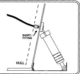
Alternate length pipe nipples: Lengths of 2-1/2', 4" and 5" are available. (Standard pipe nipple length is 3".)
