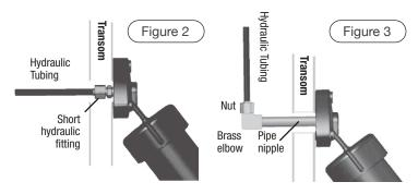
$\mbox{\bf Step 2}$  - Outside the transom, unscrew and remove the actuator away from the transom. Remove the pipe nipple.
