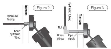
**Step 2** - Outside the transom, unscrew and remove the actuator away from the transom. Remove the pipe nipple.
