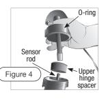
Screw the new upper hinge onto the cylinder while keeping the sensor rod inserted into center of the piston (Figure 4). Tighten the upper hinge as tight as you can by hand. You will finish tightening the cylinder in Step 7.
