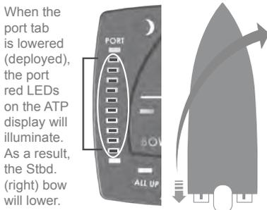
The red LEDs represent the actual movement of the tabs. As the tabs move from the full-up position to the full-down position the red LEDs will illuminate to illustrate the trim tab
