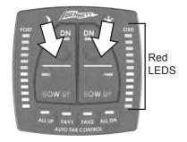
8. Press and hold both BOW UP buttons until both actuators return to the full-up position. The red LEDs on the display should show the actuator position as the actuators retract.
