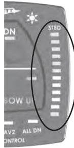
AutoTrim Pro is equipped with tab position indication LED indicators. For this feature to work, actuator sensors must be present.
