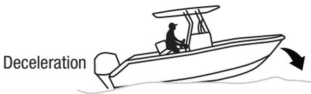
The ATP will monitor the speed over ground from the GPS and sense a deceleration and the associated bow rise as a boat is decelerating and coming off plane. The ATP controller will fully deploy the trim tabs when it senses this condition to minimize the amount of bow rise associated with
