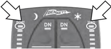
detect the presence of sensors in the actuators. Check to make sure the red and green banded sensor cables are connected to the ATP Control Unit. If the system does not have actuator sensors, skip to pg. 22.
