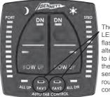
These two LEDs will flash alternately to indicate the system senses rough sea conditions.
