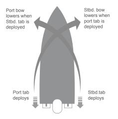
meaning the port (left) trim tab controls the starboard (right) bow. Conversely, the starboard (right) trim tab controls the port (left) bow.
