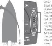
When the Stbd. tab is lowered (deployed), the Stbd. red LEDs on the ATP display will illuminate. As a result, the port (left) bow will
