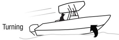
navigates a desired course. As a boat turns, the changing water flow under the vessel will cause the pitch and roll attitude of the vessel to change while the boat is in a turn. As soon as the vessel exits the turn, the boat's attitude will return to normal. Turns during operation of a boat are a very temporary condition. For this reason
