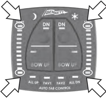
7. Press and hold both BOW DN buttons until both actuators fully extend. The red LEDs on the display should show the actuator position as the actuators deploy.
