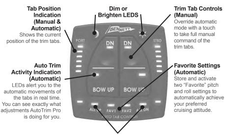
Tabs "All Up" or "All Down" (Semi-automatic) Fully retract or deploy tabs with a single touch whenever needed
