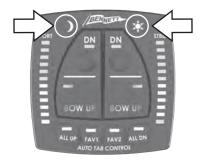
simultaneously for about three seconds. The upper yellow lights should stop flashing and all of yellow LEDs in the corners should be illuminated. These steps cannot be completed until the boat is launched and in the water.
