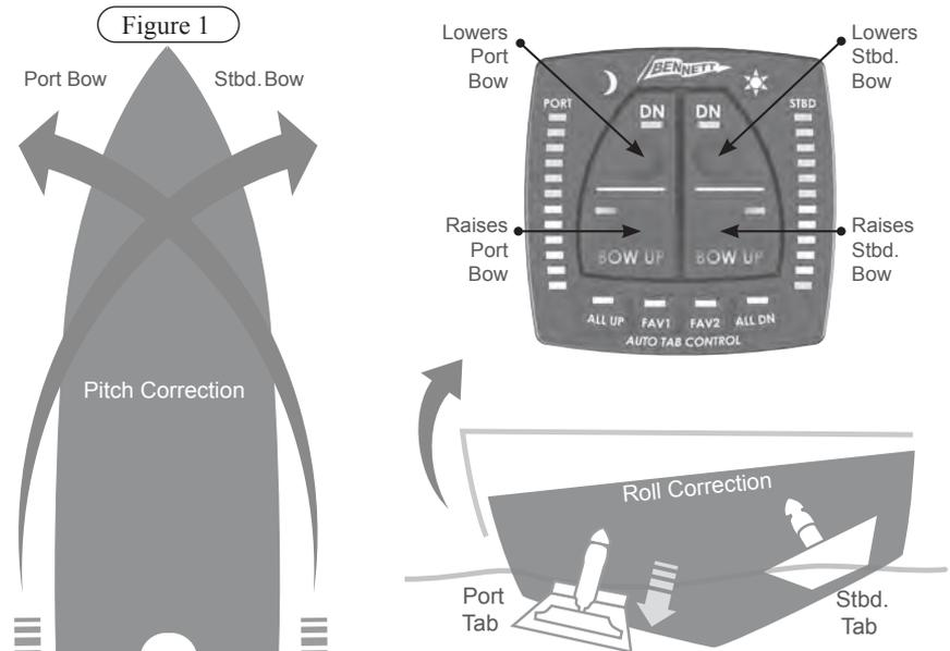
When the port tab is lowered independently, an upward force at the port stern of the boat is created. The inverse applies when lowering the stbd. tab independently.
