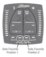
The ATP Helm Display allows for the user to set two different favorite positions. These positions are a combination of pitch and roll attitudes that the user feels are comfortable or useful running attitudes for the boat.
