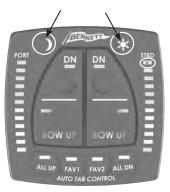
The Sun and moon buttons are used to increase and decrease the brightness of the LEDs on the display.
