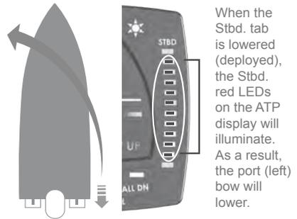
No red LEDs illuminated indicates that the tabs are fully retracted (up). If the red LEDs are flashing, the system does not have a calibration stored for the position display. See pg. 20 for calibration instructions.
