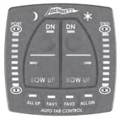
These LEDs represent the range of motion that the trim tabs may move through. The four vellow LEDs will be illuminated continuously during normal operation. If one of the upper vellow LEDs is flashing, this is an indication to the user that the system is not receiving a signal from one of the actuator sensors (see pg. 20).
