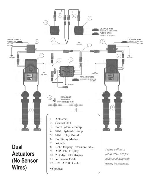
**Please note:** Trim tab position indication will not work with this setup. See pg. 10 for setup with indication. To add sensors see BennettTrimTabs.com/ATPSensors
