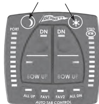
The Sun and moon buttons are used to increase and decrease the brightness of the LEDs on the display.
