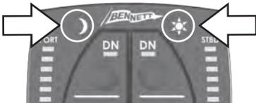
simultaneously for about three seconds. This will enter the system into calibration mode. The lower two yellow LEDs should begin to flash.
