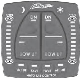
These LEDs represent the range of motion that the trim tabs may move through. The four yellow LEDs will be illuminated continuously during normal operation. If one of the upper yellow LEDs is flashing, this is an indication to the user that the system is not receiving a signal from one of the actuator sensors (see pg. 20).
