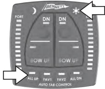
The system will flash all four corner LEDs to indicate that a setting has been made.
